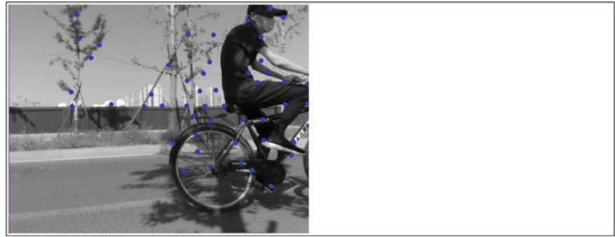
Fig. 7 Visual feature points fail because of a moving object in the camera view, there is nothing in the residual plot compared with Fig. 5
