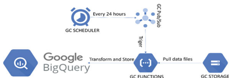
Fig. 6 Transformation and storage (analytics and visualizations) of data pipeline
